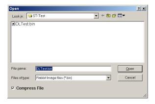
Select either a DC or SofTools .bin file. The "Compress File" option should be checked. This will compress the file and then transfer it to the board. If no file is marked "Primary" this file will automatically be marked primary.
