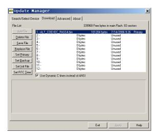
The download tab displays the files for the selected board. There are 12 file slots. Files can be marked as "Primary", "Backup", "Init" or "Unused". When the DLM boots, it will try to run the Init file, then primary file. If that fails or is corrupted, it will run the backup.
