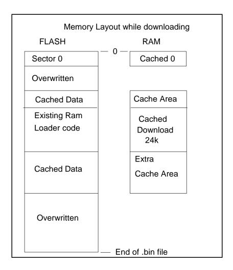
When the downloader is run, the Ram loader is copied from FLASH to RAM and then run. The existing parameters are passed to this program. Note: The FLASH is not erased and only areas specified as part of the bin file are overwritten. This assures that any user FLASH areas are preserved (i.e. a file system.).
