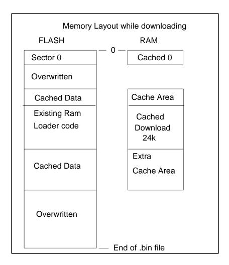
When the downloader is run, the Ram loader is copied from FLASH to RAM and then run. The existing IP and location in FLASH is passed to this program. Note: The FLASH is not erased and only areas specified as part of the bin file are overwritten. This assures that any user FLASH areas are preserved (i.e. a file system.).
